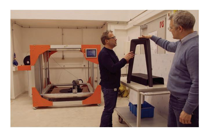
With the BigRep ONE, Steelcase produces functional, full-sized models up to 90% faster than before. The company demonstrated with a seat shell prototype that's able to bear a user's full weight they printed in just four days on their large-format 3D printer. Alternatively, producing this quality prototype with traditional methods would have taken around two months at significantly more expense. While the same form could be produced using smaller glued-together prints from a desktop 3D
