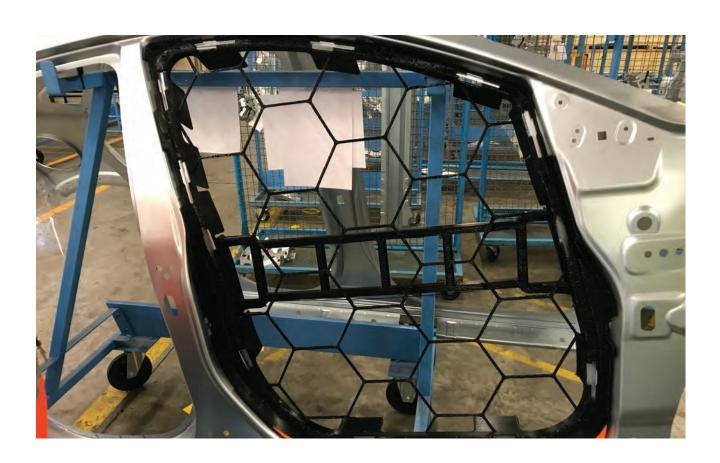
Before investing in large-format additive, Ford's welding fixtures had to be manufactured from metal in a highly manual machining process. Ford requires about 190 fixtures for a single prototype – without any potential for reuse – and lead times for machined fixtures were often as long as 3 weeks. The process
